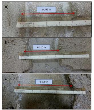
**Fig. 4:** Lateral movement W when flow rate Q is 0.36 L/s at (a)  $\beta$  is 60 degree, (b)  $\beta$  is 80 degree and (c)  $\beta$  is 90 degree
