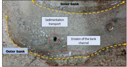
**Fig. 3:** Erosion at the bank channel of  $M_3$  with angle of direction  $\beta$  is 90 degree
