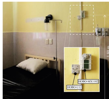
Fig. 3: Measurement instruments for Winter in Room 03.
