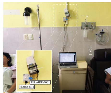
Fig. 4: Measurement instruments for Summer in Room 03.
