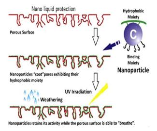
Fig. 1: Performance of nano-liquid on the mortar surface
