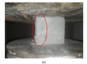
**Fig. 5:** (a) Failure pattern of 28 dayslime curing (5ml) coated (b) Failure pattern of lime curing (5ml) non-coated
