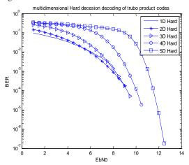
Fig. 5: Multidimensional turbo product codes for hard decision decoding
