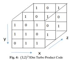
The calculation of a syndrome in different directions is based on the dimension of the product code for the dimension applying a parity check operation in the yz direction, where as the y direction syndrome is calculated by a parity check operation in the xz direction
