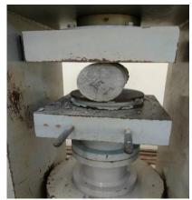
Fig. 4: Split tensile strength test
