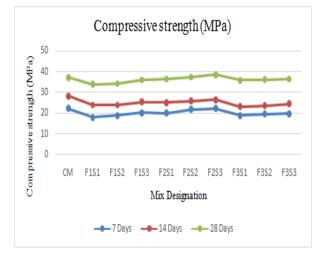
Fig. 5: Variation in compressive strength (MPa).
