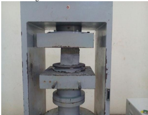
Fig. 3a: Test on Compressive strength of cube specimens
