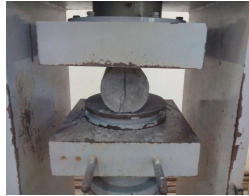
Fig. 3b: Test on split-tensile strength of cylinder specimens
