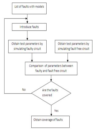
Fig. 2: Flow chart on OBIST method for testing Procedure
