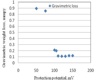
Fig. 5: Evaluation of CP criterion for cathodic protection of steel in chloride free concrete slab
