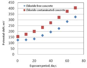
Fig. 3: Potential shift-time profile for galvanically protected concrete slab
