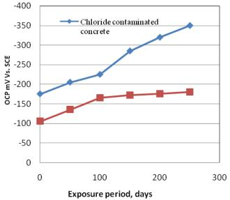
Fig. 1: Potential-time behaviour of embedded steel in concrete slab
