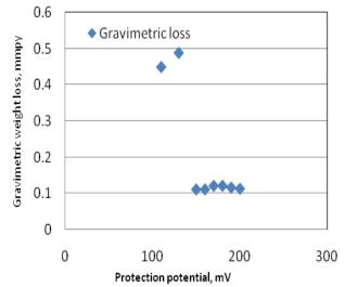
Fig. 4: Evaluation of CP criterion for cathodic protection of steel in chloride contaminated concrete slab
