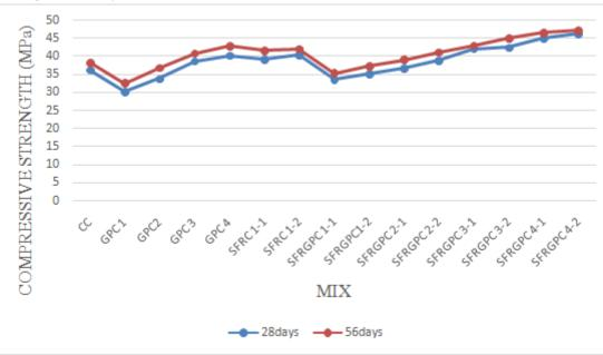
Fig. 1: Compressive strength test results
