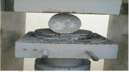
Fig. 2: Splitting tensile strength test setup
