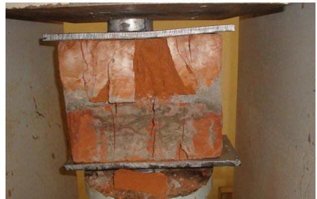
Fig. 2: Experimental set-up of compressive testing
