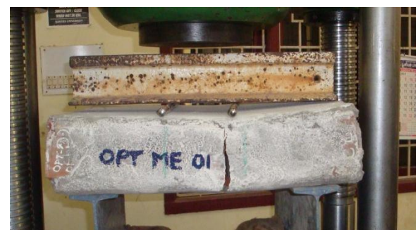
Fig. 3: Experimental set-up of EM masonry panel out-of-plane loading
