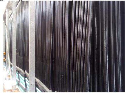
**Fig. 4:** The cross-flow plastic condenser of the Oman SWGH.
