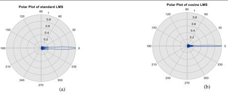
Fig. 5: Polar Plots of standard LMS and cos-LMS
