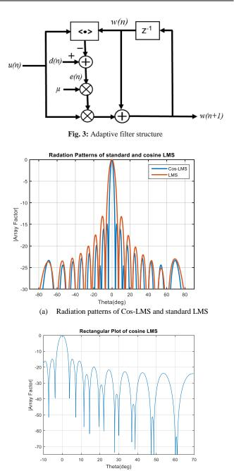
(b): Radiation patterns of Cos-LMS showing deeper null placement (below -75 dB) when interferer is at 60<sup>0</sup>
