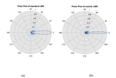
Fig. 7: Polar Plots of standard LMS and cos-LMS for 8 elements array
