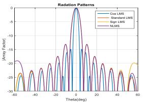
Fig 9: Radiation patterns of Cos-LMS,S-LMS, Standard LMS and N-LMS
