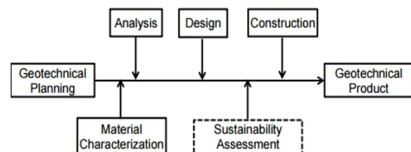
Figure 1. Processes of Geotechnical Engineering
