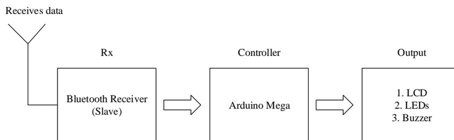
Figure 2: Block diagram of sensor node
