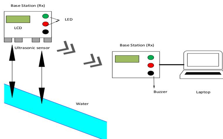
Figure 3: Flood monitoring system setup
