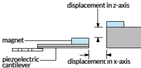
**Figure 1:** A schematic diagram of piezoelectric energy harvester in axial displacement for x-axis and z-axis.
