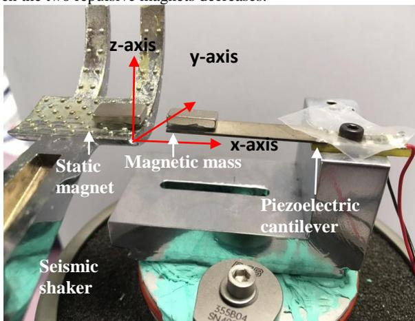
**Figure 2:** Layout of experiment apparatus and its respective axial displacement labelled accordingly.
