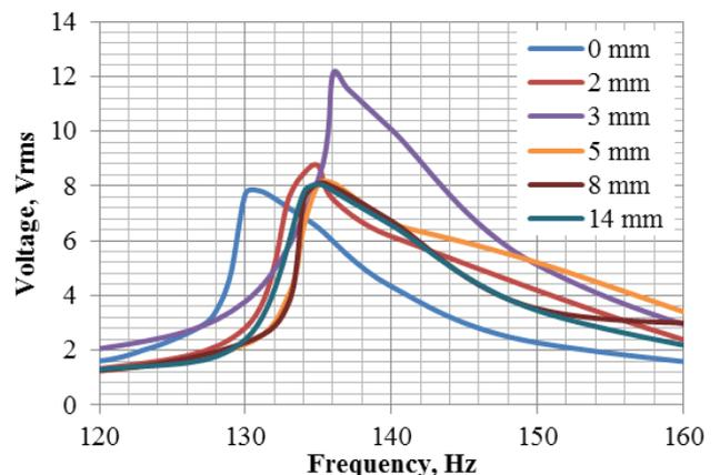
**Figure 6:** Frequency response curves of the open circuit voltage of the energy harvester for different values of z-axis displacement at horizontal displacement of x = 6 mm.
