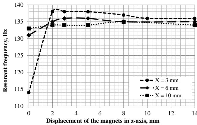
**Figure 4:** Deviations of the resonant frequency of the energy harvester as a function of z- axis displacement for x= 3 mm, 6 mm and 10 mm displacement in the x-axis.
