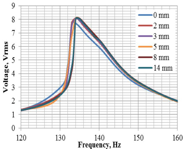
**Figure 7:** Frequency response curves of the open circuit voltage of the energy harvester for different values of z-axis displacement at horizontal displacement of  $x = 10$  mm.
