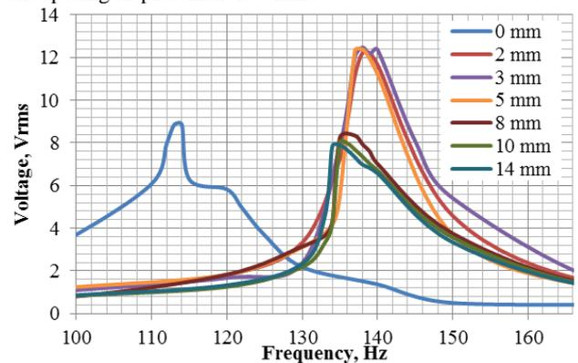
**Figure 5:** Frequency response curves of the open circuit voltage of the energy harvester for different values of z-axis displacement at horizontal displacement of x = 3 mm.
