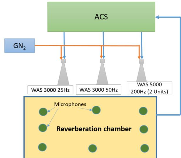
Figure 2: Configuration of RATF Close Loop Acoustic Control System
