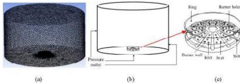
Figure 2: (a) computational domain, (b) boundary conditions and (c) burner head (upper plate and ring)
