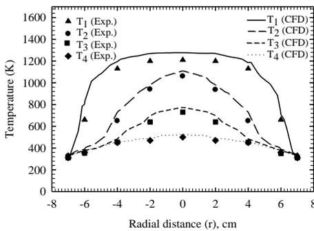
Figure 4: Temperature distribution obtained from experiment and CFD model.
