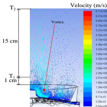
Figure 6: Velocity field at the burner head in the mid-plane.
