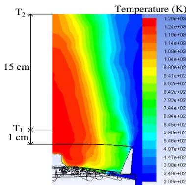
Figure 5: Temperature distribution at the burner head in the mid-plane.
