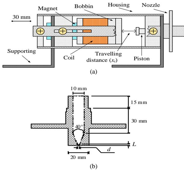
**Figure 1:** (a) Electromagnetic actuator for needle-free jet injection and (b) Nozzle
