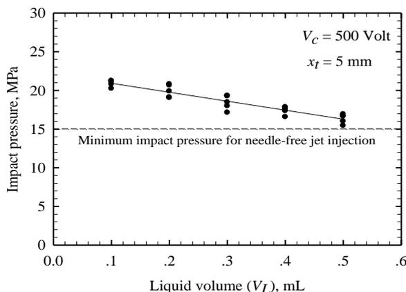
**Figure 6:** Effect of liquid volume on impact pressure at 500 Volt.
