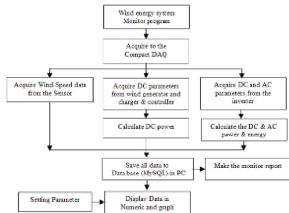
Figure 3: Diagram of LabVIEW based monitor program for WTES
