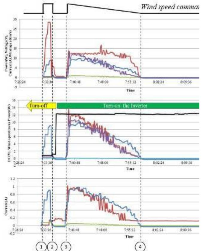
**Figure 5:** Real time output of MWT (on-grid system) by the Data Morning system via LabVIEW
