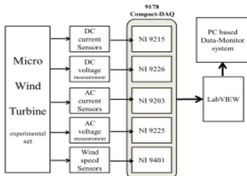
Figure 1: Diagram of the signal sensor and data acquisition module for MWT experimental set via LabVIEW
