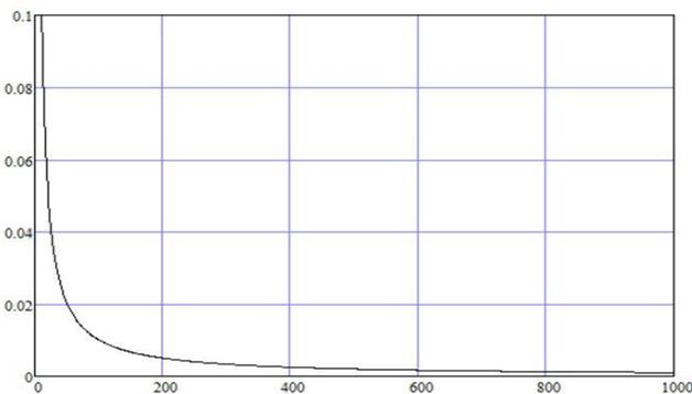
**Fig.3:** The probability of detection of false results in a decentralized multiagent system with two attackers depending on the number of agents in the system M.
