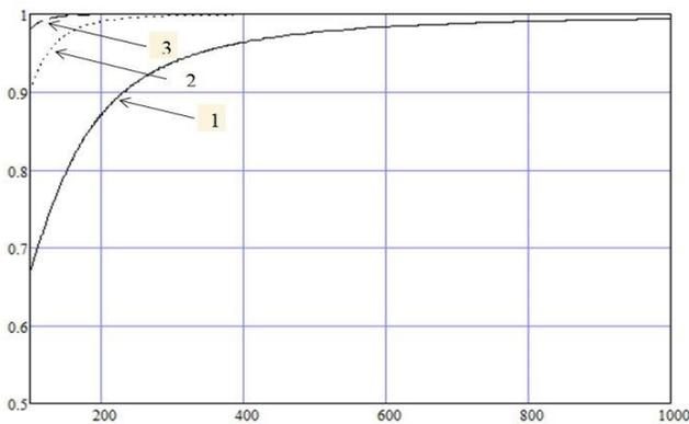
**Fig.2:** The probability of not detecting 1) one 2) two or 3) three false results in a centralized multiagent system with one managing agent.
