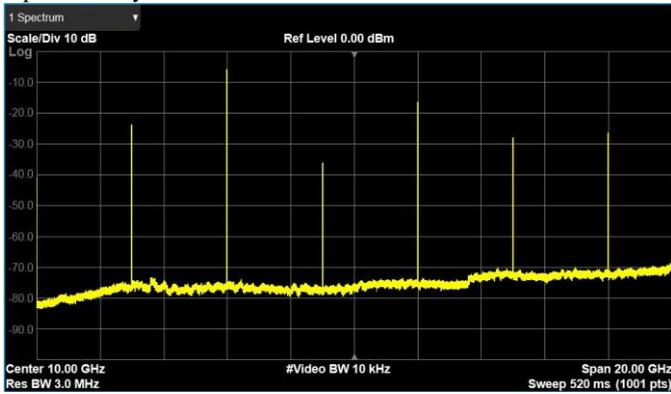
Fig. 2. Spectrum of the signal at the output of the frequency multiplier on the LTC 5553 chip with a power divider, at  $P_{in} = 10$  dBm;  $f_{in} = 3$  GHz.
