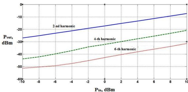
Fig. 3 - Amplitude characteristics in the mode of frequency multiplication for three even harmonics Divider of power is the equal-arms.
