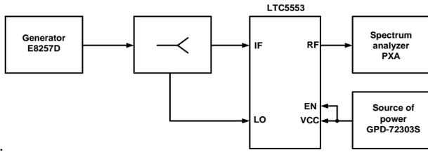
Fig. 1. Block diagram of a measuring installation with a equipotential power divider
