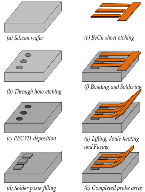
Figure 3: BeCu probe array fabrication.
