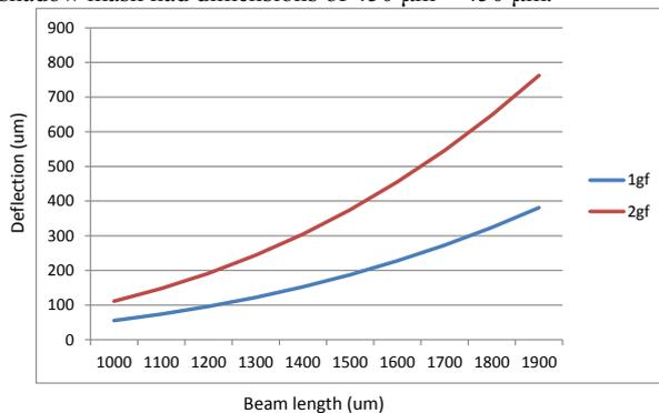
Figure 2: Deflection of the probe beam as a function of its length.
