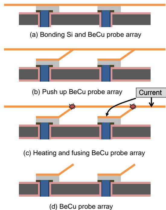
Figure 4: Bonding between BeCu and silicon substrate and formation of BeCu probe array using heat and fusing currents.
