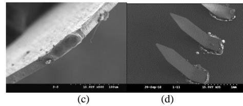
Figure 6: Fabricated probe array. (a) Optical image. (b) and (c) SEM images of cutting planes with designed dimensions of (b) 70 μm × 15 μm and (c) 50 μm × 15 μm. (d) SEM image of the fabricated BeCu probe array.
