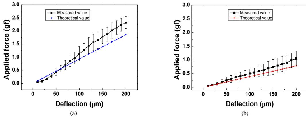
Figure 8: Contact force as a function of deflection for beam lengths of (a) 1.7 mm and (b) 2.1 mm.
