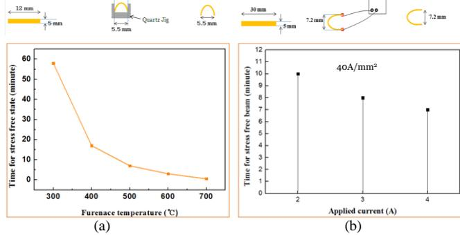
Figure 5: Comparison of the stress relaxation of a BeCu beam heated by (a) a furnace and (b) an applied current.
