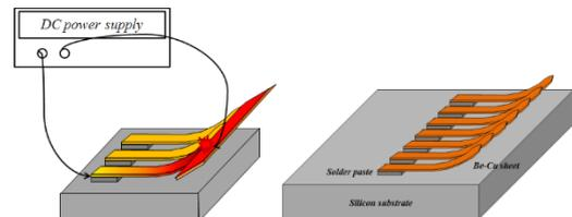
**Figure 1:** Formation of the proposed BeCu probe array using heat and fusing currents.
