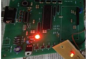
Fig. 6: LED Blinking in PIC Board
