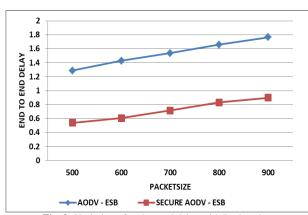
Fig. 9: Variation of end to end delay with Packet size
