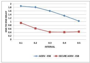
Fig. 5: Variation of end to end delay with different Interval
