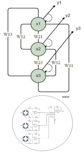
Fig. 3: Proposed memristive Hopfield neural network
