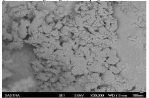
Fig.1 : SEM microstructure of nano silica
