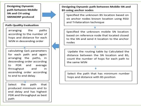
Fig. 2: Illustrate Study Method Functional Diagram.
