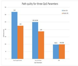
**Fig. 5:** The Network Performance is Improved when Using Mobile SN Because It Gives Lowest Delay Value and Total Dropped Packets in Compare with Using Static SN.
