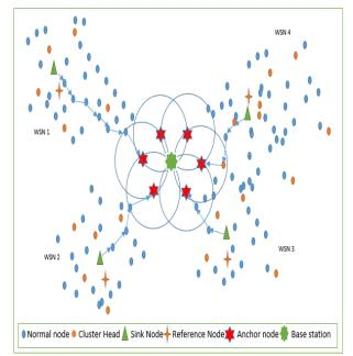
Fig. 1: The Network Framework Consisted of Four WSN with Four Mobile Sink Nodes connected to six Anchor Nodes around Single BS, Four Reference Nodes Specified the Mobile Sink Node Location. Blue Arrows Represented the Designing Path.
