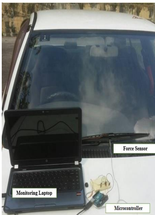
Fig. 5: Setup for contact force measurement.
