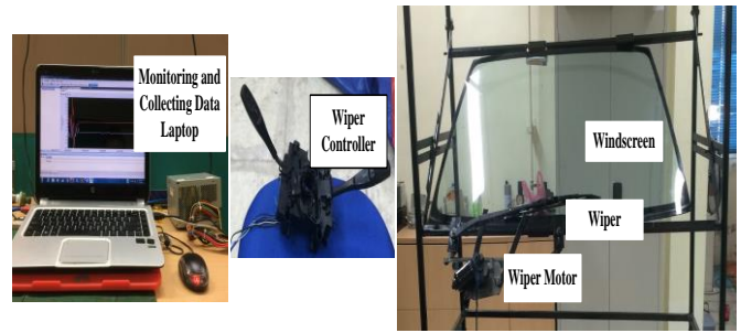
Fig. 2: Wiper system experimental rig
