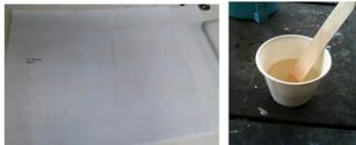
Fig. 1: Plain woven Bombyx mori silk fibre and epoxy resin.
