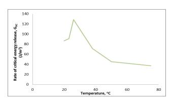
Fig. 8: Graph of Mode II interlaminar fracture toughness for each specimen for ENF test.
