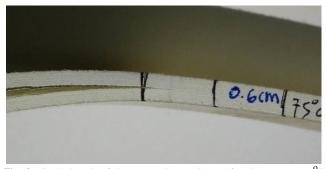
**Fig. 9:** Crack length of the composite specimen after the test at 75  $^{\circ}$ C which is at 6 mm from the pre-cracked point.
