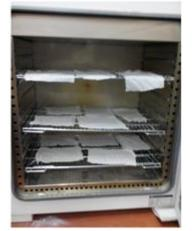
Fig. 3: Treatment of silk fibre with silane coupling agent and ethanol inside an oven.
