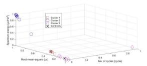
Fig. 9: Three clusters for normalised number of cycles, normalised RMS and normalised energy using k-means clustering approach in 3D
