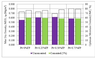
Fig. 4 :MDD-OMC of uncemented & cemented reinforced peat with fiberpolyester (FP)
