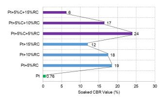
Fig. 10: Effect of inclusion of shredded rubber-crumb on soaked CBR value
