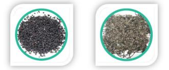
Fig. 2: Processed tire-waste disposal: (a) Shredded rubber-crumb and (b) Fiber-polyester
