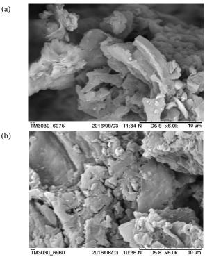
Fig. 9: SEM image (a) Uncemented peat at 28 days X40 (b) Cemented peat at 28 days X40
