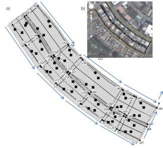
Fig. 6: Scenario 1, a) Modelling of existing drains, b) Existing drains and direction of flow
