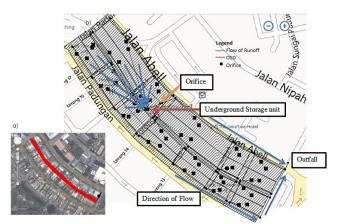
Fig. 7: Scenario 2, a) Location of OSD1, and b) Inclusion of OSD1
