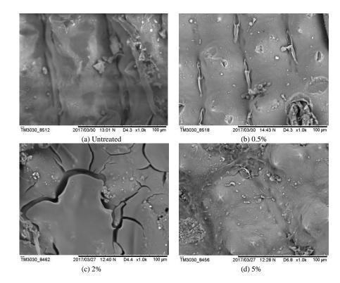
Fig 1: SEM images of the untreated and silane treated rice husk
