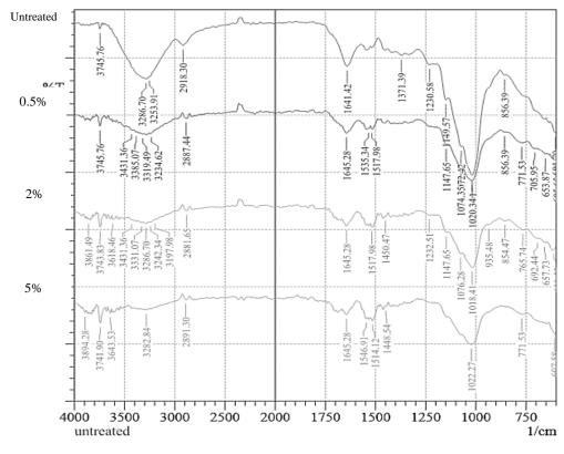
Fig 2: FTIR spectra of untreated and silane treated rice husk
