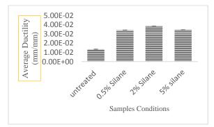
**Fig 5:** Effect of silane treatment on average ductility of rice husk/phenol formaldehyde particleboard
