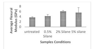
Fig 4: Effect of silane treatment on average flexural modulus of rice husk/phenol formaldehyde particleboard
