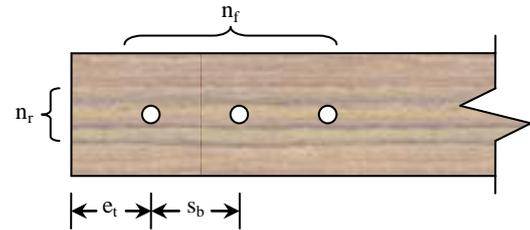
Fig. 1: Variables of timber bolted connections
