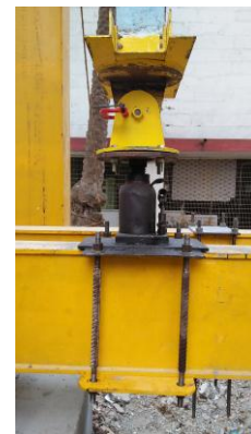
Fig 7: Hydraulic Jack arrangement for the axial load to the column
