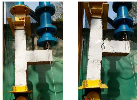
Figure 9: Ductile Specimen Before and After Testing
