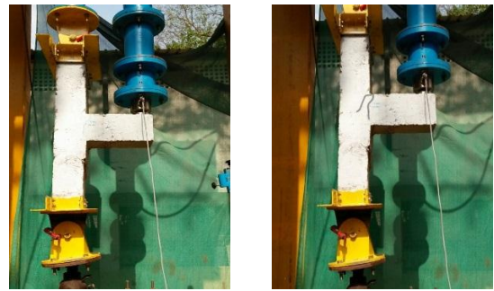
Figure 8: Control specimen before and after testing
