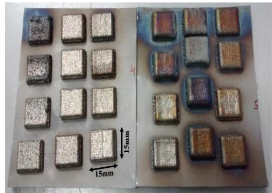
Fig. 2: LENS deposited Co-Cr-W alloy samples
