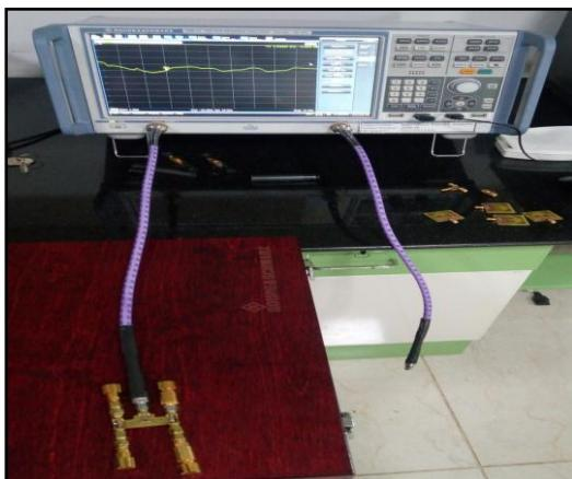
Fig. 14: Testing arrangement of proposed 1X4 power Divider on FR4 Material
