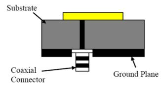
Fig. 2: Coaxial Probe Feed Technique
