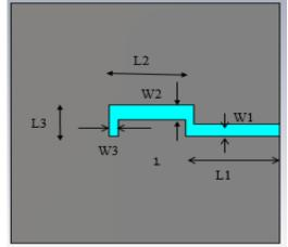
Fig. 4: Design of U slot antenna
