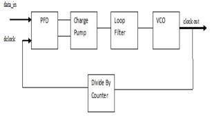
Fig. 1: Phase Locked Loop
