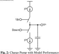
Method of the charge pump possibly tabularized and it is the ultimate action of pump. It describes the controls of the charge pump. It charges or releases the present of the pump associated with rate of error sign (pulse width of the RISE or DOWN) created by the Phase Frequency Detector. The actions are listed in table.1.
