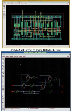
Fig. 7: Schematic circuit of Phase Detector
