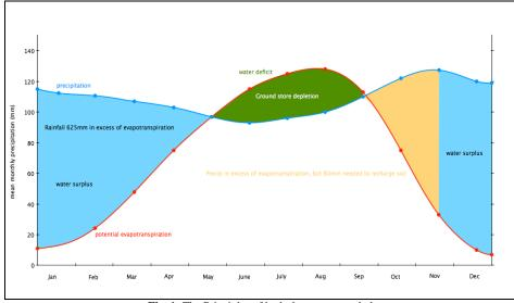
Fig. 1: The Principles of hydrology on water balance concept
