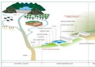
Fig. 1: Typical drinking water supply system in Malaysia
