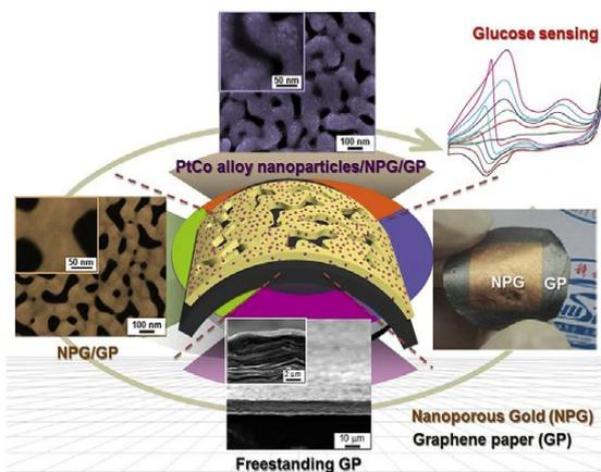
Fig. 2: Free standing, flexible GP and NPG electrodeposited with PtCo for nonenzymatic biosensor in [8].
