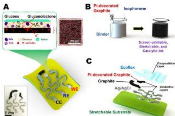
Fig. 1: Design of stretchable screen printed biosensor using Pt-graphite ink onto flexible PU as in [7]. Preparation method is simple and low cost.
