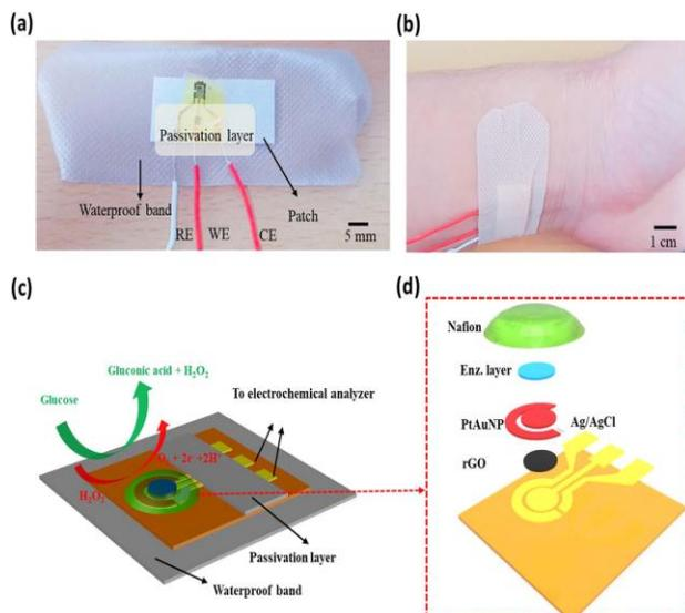
**Fig. 6:** Image of patchable sweat based glucose biosensor in [17].
