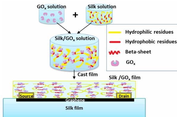
Fig. 3: Stabilized graphene/FET on biocompatible silk film in free standing, flexible GP and NPG electrodeposited with PtCo for nonenzymatic biosensor in [10].
