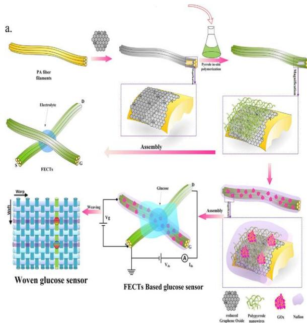
**Fig. 5:** Preparation of woven fiber organic electrochemical FET using PA fiber in [13].
