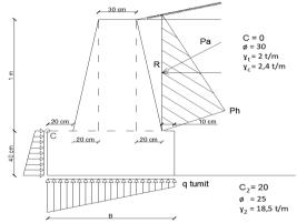
Fig 4: Dimension of Retaining Wall
