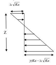
Fig 1: Active Soil Pressure Rankine
