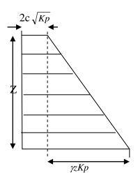
Fig 2: The Pressure of a Passive Rankine
