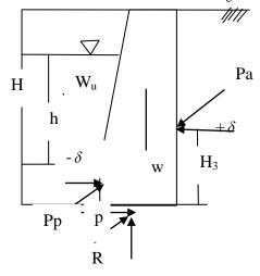
Fig 3: Ground-Style-Wall-Retaining Wall
