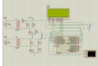
Fig 4: Harmonic Meter Circuit
