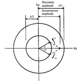
Fig 2: Contra-rotating vector pair producing a varying amplitude (pulsating) vector
