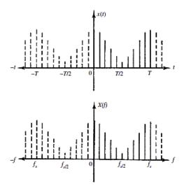
Fig 2: Discrete time- and frequency-domain function
