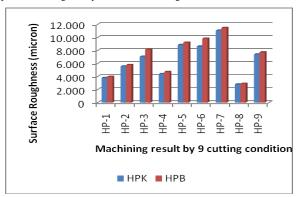
Fig 7: Relation of surface roughness with 9 cutting conditions at dry and wet machining
