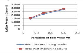
Fig 6: Surface roughness as a function of Variation of tool wear for optimum cutting on dry and wet machining
