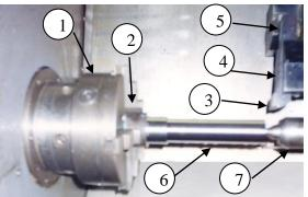
Fig 1: Workpiece installed on CNC lathe machine
