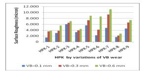
Fig 4: Surface roughness as a function of Variation of VB wear for dry machining
