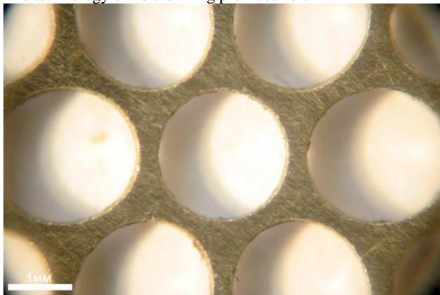
**Fig 2:** The back side of samples from titanium alloy OT4-1 obtained by drilling on the CNC machine MANO 500 before the deburring and rinsing.
