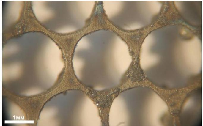
**Fig 3:** The front side of the holes on titanium alloy OT4-1 sample with the thickness of 0.5 mm obtained on a laser device "Bystar 3015". A continuous operation mode made 30% of rated power. The speed made 5000 mm/min, the gas pressure made 6 bar.
