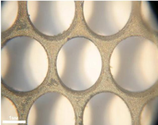
**Fig 1:** The front side of the holes on titanium alloy OT4-1 sample with the thickness of 0.5 mm obtained by the "super drill" method using Anchem HSD6-II unit.
