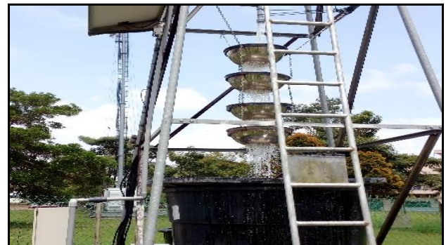
Fig. 3: Water-into-air aeration method (fountain)
