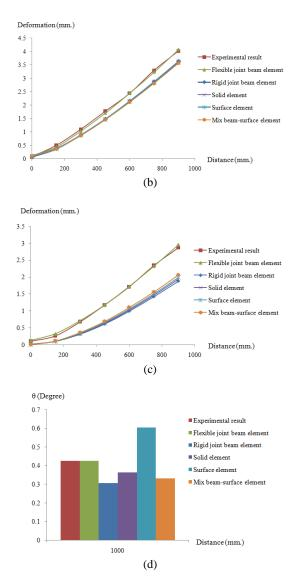
Fig. 7: The result of beam deformation in different element types respected to the experimental result; (a) Applied load on X-axis, (b) Applied load on Y-axis, (c) Applied load on Z-axis, (d) the angular deformation when applied bending moment on X- axis.
