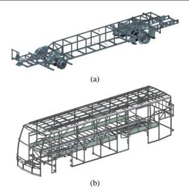
Fig. 1: Bus superstructure; (a) Chassis frame, (b) Body structure.
