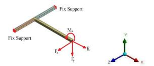
Fig. 3: FE model of T-junction beam including the boundary condition.
