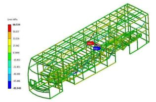
Fig. 8: Maximum stress distribution occurred on the body structure in a case of torsion load.
