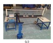
**Fig. 4:** The each direction of applied load on T-junction beam including the digital dial gauge; (a) X-axis, (b) Z-axis, (c) Y-axis.
